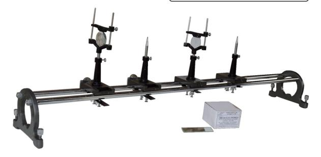
**OMEGA TYPE ES-298** Experimental Set-Up has been designed specifically to find the focal length of a convex mirror using (1) plane mirror (2) convex lens.
