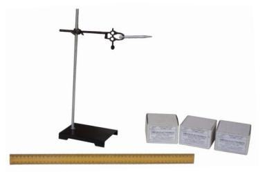
OMEGA TYPE ES-299 Experimental Set-Up has been designed specifically to determine the refractive index of a liquid using a Concave Mirror.
