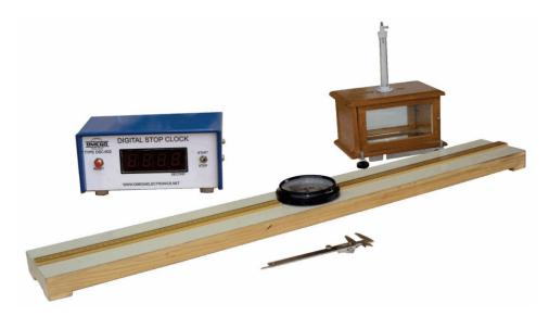
OMEGA TYPE ES-305 Experimental Set-Up has been designed specifically to determine the Horizontal Component of Earth's Magnetic Field B<sub>H</sub>and the Magnetic Moment M of the Magnet bar using Deflection and a Vibration Magnetometers.
