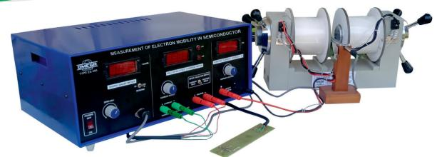
OMEGA TYPE ES-306 Experimental Set Up has been designed specifically for the Measurement of Electron Mobility in Semiconductor (Drift velocity of the charge carrier acquired per unit electric field) and Hall Co-efficient. The set-up consists of Electromagnet, Constant Current Power supply, Digital Gauss Meter, Hall Effect Board, Hall Probe (Ge crystal n-type) with stand.
