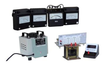
**OMEGA TYPE ES-308** Experimental Set-Up has been designed specifically to find the Voltage & Current relationship in a R-L series circuit and to determine the Power Factor of the circuit. The set-up consists of Voltmeter, Ammeter, Wattmeter, Variac, Inductor and Fixed resistance in three steps.
