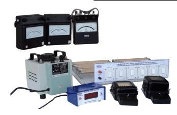
**OMEGA TYPE ES-309** Experimental Set-Up has been designed specifically to find percentage error in a single phase energy meter. The set-up consists of two Energy meters, Wattmeter, Voltmeter, Ammeter, Variac, Digital stop clock and Variable load.
