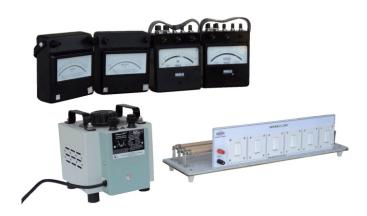
**OMEGA TYPE ES-310** Experimental Set-Up has been designed specifically to measure the power and power factor in a single phase A.C. circuit. The set-up consists of Voltmeter, Ammeter, Wattmeter, Power factor meter, Variac and Variable load.
