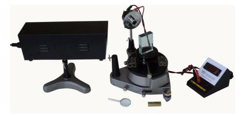
**OMEGA TYPE ES-312** Experimental Set-Up has been designed specifically to study the Polarisation of Light by Simple reflection using Laser. The set-up consists of Circular table, Diode Laser, Glass Slab, Analyser attachment with Laser Detector, Nanoammeter, Reading lens and Spirit Level.
