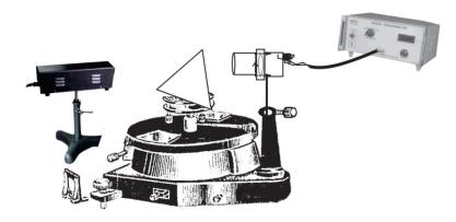
**OMEGA TYPE ES-313** Experimental Set-Up has been designed specifically to determine Brewster's angle for a glass prism surface and hence to determine refractive index of glass using Laser. The set-up consists of Circular table, Diode Laser, Glass prism, Laser Detector, Nano-ammeter, Reading Lens and Spirit Level.
