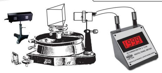
**OMEGA TYPE ES-314** Experimental Set-Up has been designed specifically to determine the Refractive Index of liquids (Water, Paraffin Oil, Glycerol, Kerosene, Benzene etc.) in the form of prism by using Laser and it's detector. The set-up consists of Circular table, Helium Laser, Hollow Prism, Laser Detector, Digital Milliammeter, Reading lens and Spirit Level.
