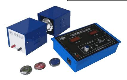
**OMEGA TYPE ES-317** Experimental Set-up has been designed specifically for determination of Planck's constant by Vacuum type Photo Cell with three filters.
