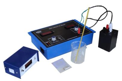
OMEGA TYPE ES-321 Experimental Set Up has been designed specifically for determination of Heat capacity of Solids. The experimental set-up is self contained and require no other apparatus.
