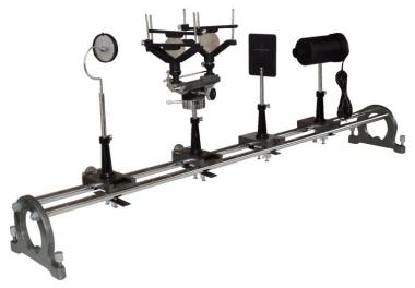
**OMEGA TYPE ES-322** Experimental Set-Up has been designed specifically for determination of focal length of a combination of two convergent lenses using Nodal Slide Assembly. The set-up consists of Nodal Slide Assembly, Light s ource, optical screen, plane mirror & convex lens.
