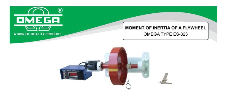
**OMEGA TYPE ES-323** Experimental Set-Up has been designed specifically for determination of Moment of Inertia of a Flywheel about its own axis of rotation. The set-up consists of Flywheel Digital stop clock, vernier callipers & set of weights.
