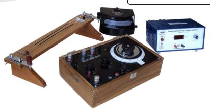
OMEGA TYPE ES-325 Experimental Set-Up has been designed specifically for measurement of low resistance of cables, conductors in industries or laboratory. The set-up consists of Industrial Kelvin Double Bridge, Conductivity Attachment for Industrial Kelvin Double Bridge, Spot Reflecting Galvanometer, Constant Current Power Supply etc.
