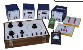
**OMEGA TYPE ES-326** Experimental Set-Up has been designed specifically to measure EMF & unknown resistance by Crompton Potentiometer. The set-up consists of Crompton Potentiometer, Cell Eliminator, Digital Electronic Standard Cell, Digital Electronic Null Detector, Potentiometer Power Supply, set of unknown resistance and DC Ammeter etc.
