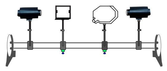
OMEGA TYPE ES-329 Experimental Set-Up has been designed specifically to compare the illuminating power of two given source of light with a Lummer Brodhum (L.B.) Photometer. The Set-up consists of Lummer-Brodhum (L.B.) Photometer, Optical Bench & two sources of light and one ground glass plate.
