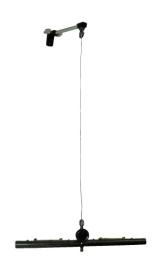
**OMEGATYPE ES-236** Experimental Set Up has been designed specifically to find the value of modulus of rigidity 'h' of material of the given wire with Maxwell's needle.
