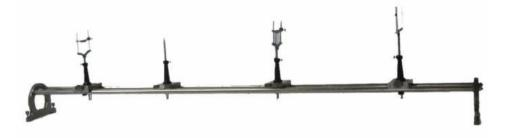
**OMEGA TYPE ES–337** Experimental setup has been designed specifically for Verification of Newton's Formula  $x_1 x_2 = f^2$  for Lenses separated by a given distance.
