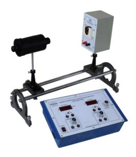
**OMEGA TYPE ES-339** Experimental setup has been designed specifically to Draw the Characteristics of a Photo Electric Cell (Vacuum Type). The experimental set-up is absolutely self contained and require no other apparatus.
