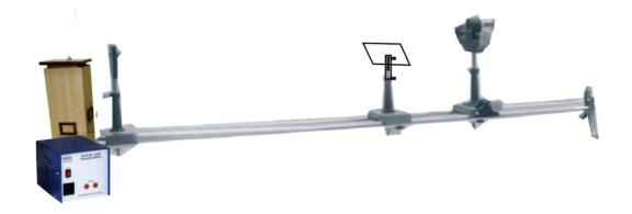
OMEGA TYPE ES-341 Experimental Set-Up has been designed specifically to determine the wavelength of monochromatic light by diffraction at a Straight Edge. The set-up consists of Optical bench with uprights, Sodium lamp, Micrometer eye piece, Optical Slit, Straight Edge (Blade) with Holder. The set-up is complete in all respect and requires no other apparatus.
