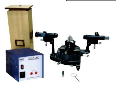
OMEGA TYPE ES-342 Experimental Set Up has been designed specifically to determine the Angle between crystal surfaces by spectrometer. The set-up consists of Spectrometer, Sodium light source, Calcitel Prism, Reading lens, Spirit Level etc.
