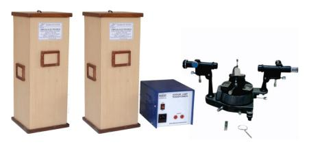
OMEGA TYPE ES-344 Experimental Set Up has been designed specifically to calibrate the spectrometer by Mercury Vapour Lamp and hence to find the wavelength of a given monochromatic source of sodium light. The set-up consists of Spectrometer, Prism, Mercury vapour lamp, Sodium light source, Reading lens, Spirit Level etc.
