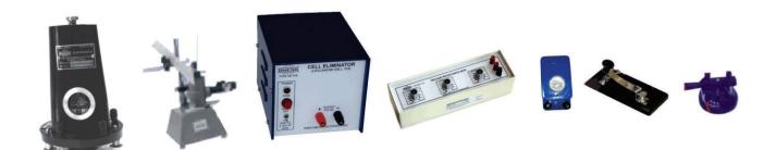
**OMEGA TYPE ES-348** Experimental Set Up has been designed specifically to Determine the Current Sensitivity and Voltage Sensitivity of a Moving Coil Ballistic Galvanometer. The set up is absolutely self contained and requires no other apparatus.
