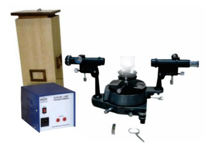
OMEGA TYPE ES-350 Experimental Set-Up has been designed specifically to determine Small Angle and Refractive Index of the Material of given Small - Angled Prism by Methods of Normal Incidence and Normal Emergence using Spectrometer. The set-up consists of Spectrometer, Mercury light source, small angled Prism, Reading lens etc.
