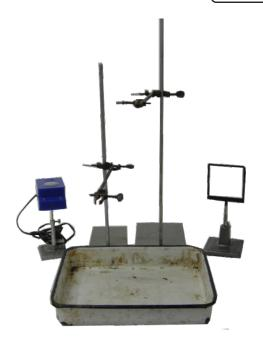
OMEGA TYPE ES-351 Experimental Set-Up has been designed specifically to determine the Refractive Index of liquids (Water, Paraffin Oil, Glycerol, Kerosene, Benzene etc.) using Laser. The set-up consists of Diode Laser, Container tray and Reflector etc.
