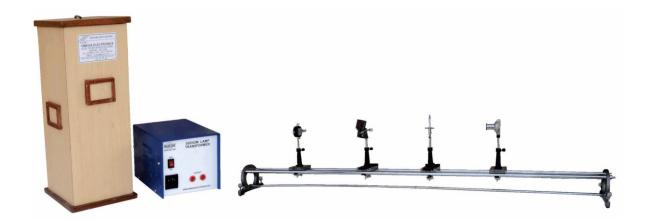
**OMEGA TYPE ES-352** Experimental Set-Up has been designed specifically to determine the Wave Length of Sodium Light Using Lioyd's Mirror. The set-up consist of Optical bench, Lioyd's Mirror, Lens Holder, Micrometer eye-piece, Optical Slit, Double Convex Lense, SOdium Light source etc.
