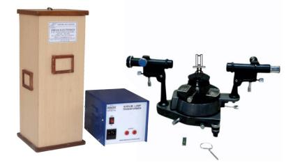
**OMEGA TYPE ES-353** Experimental Set-Up has been designed specifically to determine the Separation Between the Plates of a Fabry Perot Etalon The Set -up consist of Fabry Perot Etalon, Spectrometer, Sodium Light Source, Optical Slit, Reading Lense and Spirit Level etc.
