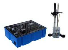
**OMEGA TYPE ES-354** Experimental Set-Up has been designed specifically for measurement of Temperature Coefficient of Resistance for Platinum, using a Callender and Griffith's Bridge, Platinum Resistance Thermometer, Galvanometer, Battery Eliminator etc.
