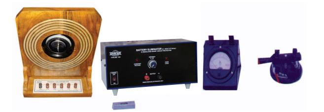
**OMEGA TYPE ES-356** Experimental Set-up has been designed specifically to study the variation of magnetic field at the center of circular coils when turns remain same and radii vary. The set-up consists of an apparatus for variation of magnetic field at the center of circular coils when turns remain same and radii vary, Battery Eliminator, Ammeter, Reversing key, Spirit level etc.
