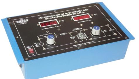
**OMEGA TYPE ES-258** Experimental Set Up has been designed specifically to determine the Hysteresis loss of a Transformer by C.R.O. The setup consists of Specimen transformer, Digital A.C. ammeter and voltmeter, Potentiometer etc.
