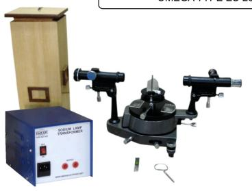
**OMEGA TYPE ES-261** Experimental Set Up has been designed specifically for the Measurement of Refractive Index of glass in the form of prism by Spectrometer. The set-up consists of Spectrometer, Sodium light source, Prism, Reading lens etc. The set up is complete in all respect and requires no other apparatus.
