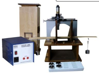
OMEGA TYPE ES-262 Experimental Set Up has been designed specifically for determination of the Young's Modulus Y of Glass by Cornu's method. The set-up consists of Traveling Microscope, Sodium light source, Screw gauge, Vernier callipers, Glass plate, Wooden platform, Glass reflector & Weights with hangers etc.
