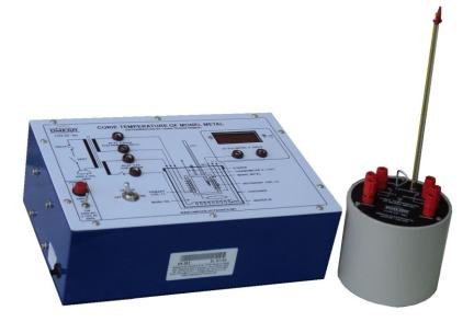
**OMEGA TYPE ES-263** Experimental Set Up has been designed specifically for determination of Curie Temperature of Monel Metal using a Transformer. The set-up consists of Monel Metal Transformer, Container, Heater, Thermometer, Stirrer etc. The set up is complete in all respect and requires no other apparatus. Practical experience on this set up carries great educative value for Science and
