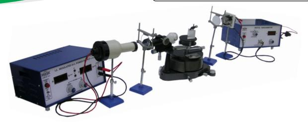
OMEGA TYPE ES-265 Experimental Set-Up has been designed specifically to study of Planck's Constant by Spectrometer and Photo voltaic cell. The set- up consists of Spectrometer, Digital Nanoammeter, Prism, Photo voltaic cell, Power supply etc.
