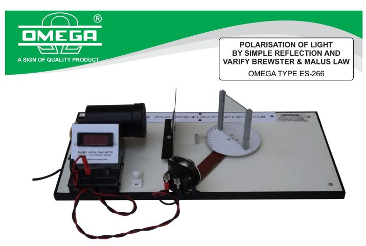
**OMEGA TYPE ES-266** Experimental Set-Up has been designed specifically to study the Polarisation of Light by Simple Reflection from a Glass Plate with the help of Nicol's Prism and Verify Brewster Law & Malus Law. The set-up consists of a Glass plate, Photo voltaic cell, Incandescent/Halogen lamp, Microammeter, Polaroid and Convex lens.
