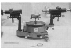
OMEGATYPE ES-267 Experimental Set-Up has been designed specifically to determine Brewster's angle for a glass surface and hence to determine refractive index of glass. The set-up consists of Spectrometer, Incandescent bulb, glass prism and Polaroid attachment to Telescope objective.
