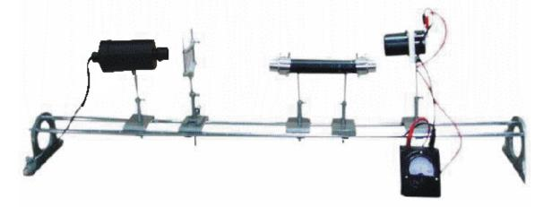
**OMEGA TYPE ES-268** Experimental Set-Up has been designed specifically to verify the Malus law (cosine square law) for plane polarised light with help of a photo voltaic cell. The set-up consists of a Optical Bench Photo voltaic cell, Halogen lamp, Convex lens, Microammeter, Polariser and Analyzer etc.
