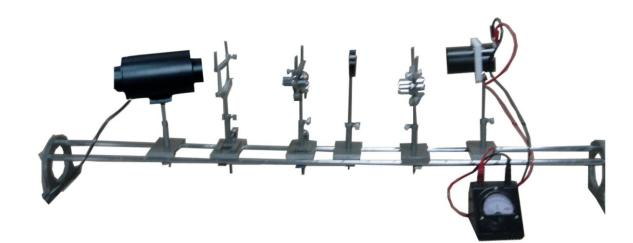
**OMEGA TYPE ES-269** Experimental Set-Up has been designed specifically for the study of Elliptically Polarised Light by means of a Photo voltaic cell. The set-up consists of source of light, Convex lens, Analysing and Polarising Polaroids, Photo voltaic cell, Microammeter, Suitable optical bench with uprights etc.
