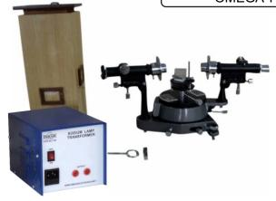
**OMEGA TYPE ES-270** Experimental Set-Up has been designed specifically to verify Fresnel's formula for the reflection of light. The set-up consists of Spectrometer, Sodium light source, Prism, A Pair of Polaroids, Reading lens etc.
