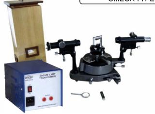
**OMEGA TYPE ES-272** Experimental Set-Up has been designed specifically to determine the Dispersive Power of a plane transmission Diffraction grating. The set-up consists of Spectrometer, Sodium light source, Diffraction Grating, Reading lens etc.
