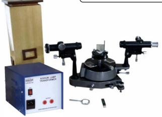
**OMEGA TYPE ES-273** Experimental Set-Up has been designed specifically to determine the refractive indices  $\mu_o$  and  $\mu_e$  of quartz prism for the ordinary and extraordinary rays using spectrometer and sodium light. The set-up consists of Spectrometer, quartz prism, Sodium light source, Reading lens etc.
