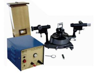
**OMEGA TYPE ES-275** Experimental Set-Up has been designed specifically for the study of Hydrogen spectrum and determination of Rydberg's constant with the help of Spectrometer, Diffraction grating and a Hydrogen spectrum tube. The set-up consists of Spectrometer, Diffraction grating, Hydrogen spectrum tube, Transformer etc.
