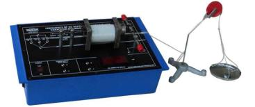
**OMEGA TYPE ES-278** Experimental Set-Up has been designed specifically to perform experiments by using Electrical Vibrator. (1) To determine the frequency of AC main by Melde's experiment. (2) To find the capacitance of a capacitor given that the frequency of AC supply is 50 cycle/sec.
