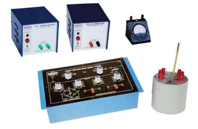
**OMEGA TYPE ES-280** Experimental Set-Up has been designed specifically to determine the temperature coefficient of resistance of conductors like copper and iron. The set up consists of P.O. Box, Galvanometer, Thermometer and Stirrer, Two conductors, Cell Eliminator, Oil bath container, etc.
