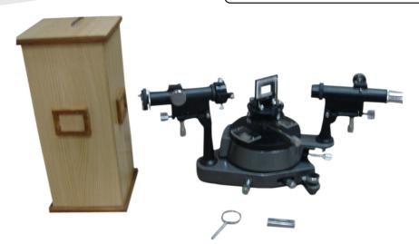
**OMEGA TYPE ES-282** Experimental Set-Up has been designed specifically to determine the Resolving Power of a Diffraction Grating. The set-up consists of Spectrometer, Mercury light source, Diffraction Grating, Rectangular Aperture of adjustable width, Reading lens etc.
