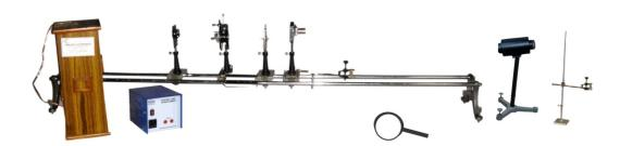
**OMEGA TYPE ES-283** Experimental Set-Up has been designed specifically for experiments with Fresnel's Bi Prism (1) To determine the wave length of sodium light (2) To determine the thickness of Mica Sheet. The set-up consists of Optical bench with uprights, Sodium light source, Bi-prism, Convex lens, Slit, Micrometer eye piece, Incandescent lamp, etc.
