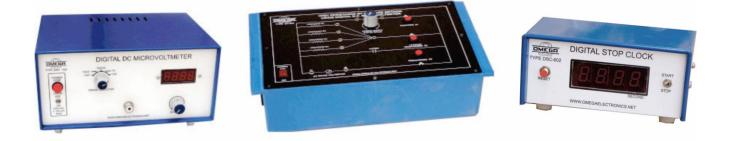
OMEGATYPE ES-286 Experimental Set-Up has been designed specifically to determine the high resistance by leakage method by means of a Digital D.C. Microvoltmeter in place of conventional Ballistic Galvanometer. The set-up consists of Digital D.C. Microvoltmeter, Tapping key, Fixed capacitor and High Megohm Resistances, Digital stop clock etc.
