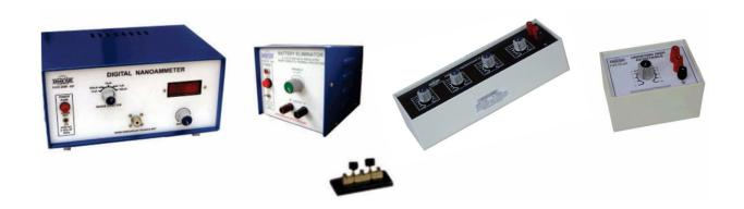
**OMEGA TYPE ES-287** Experimental Set-Up has been designed specifically for the measurement of high resistance by substitution method using Digital Nanoammeter. The set-up consists of Nanoammeter, Battery eliminator, Megohm box, Two way key etc.
