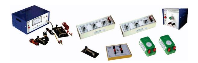
OMEGA TYPE ES-288 Experimental Set-Up has been designed specifically to compare the capacities of two condensers by the method of MIXTURES using Electronic Coulombmeter, in place of conventional Ballistic Galvanometer. The set-up consists of Electronic Coulombmeter, two resistance boxes, Battery eliminator, one double pole double throw (D.P.D.T) switch.
